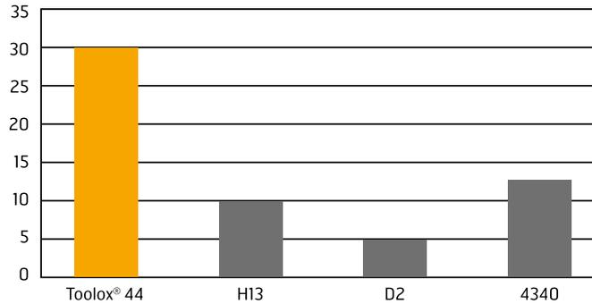
The table shows the toughness of Toolox® 44 compared to some standard steels that are heat treated to 45-55 HRC. Toughness values for Toolox® at -20°C are stated in the product certificates.
