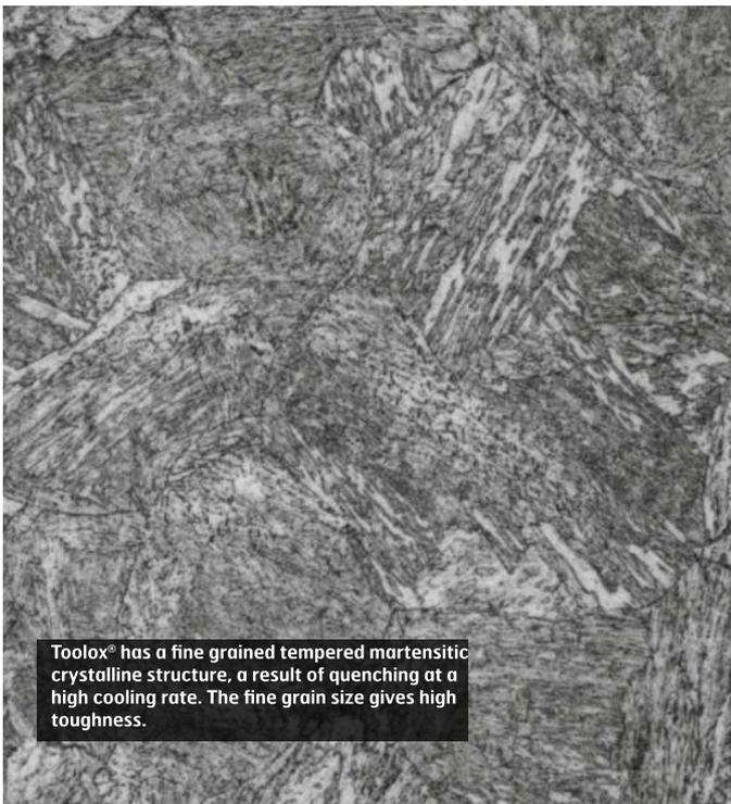
Toolox® has a fine grained tempered martensitic crystalline structure, a result of quenching at a high cooling rate. The fine grain size gives high toughness.
