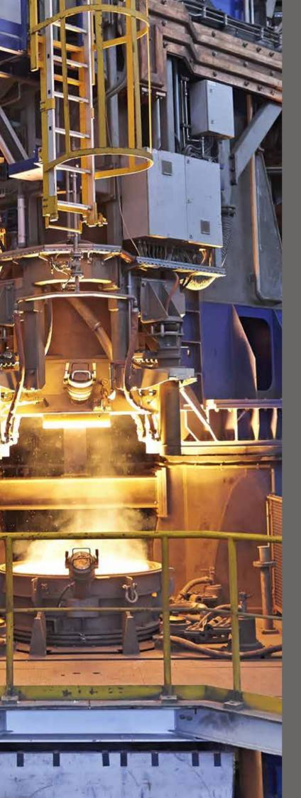
THE ELECTROSLAG REMELTING PLANT features two large 36 and 50 ton ESR furnaces and a smaller one of 3 ton. Via ESR method we can produce extra clean tool steels to ensure the maximium performance of the tool. Based on ESR remelting, we are also developing customized tool steel grades to meet requirements for even the most demanding tooling applications.
