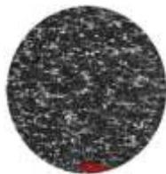
Φ263.5mm Spray Ingot Eutectic Carbide Unevenness: grade 3
