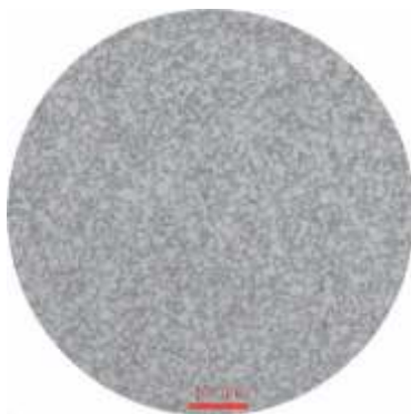
Large Grain Carbide Size : 3.5um
