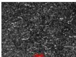
210×410mm Spray Ingot Eutectic Carbide Unevenness: grade 2
