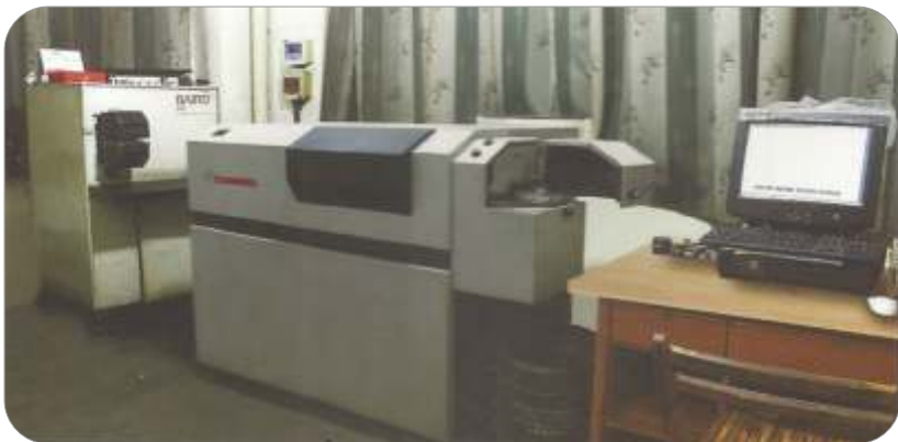
American and Swiss spectrometers content of W, Mo, Cr, V, Co, S, P, N, Nb and so on.
