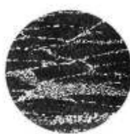
Φ280mm Mold Ingot Eutectic Carbide Unevenness: grade 5
