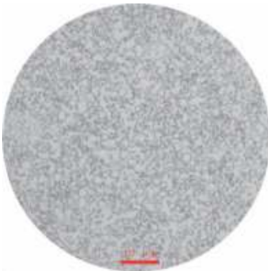
Large Grain Carbide Size : 3.5um
